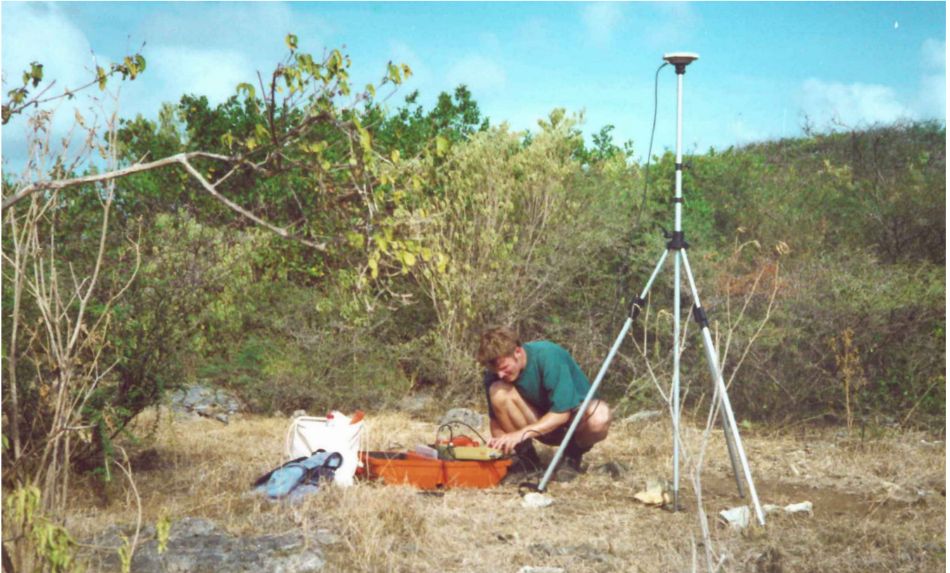
Fig. 2.6. Performing GPS measurements at the Nord Morne Zambé site, Pointe des Châteaux.
